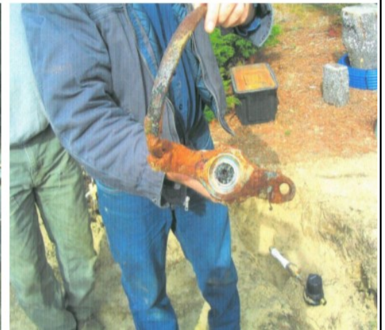
The pictures above show the water service replacements being done in Greentrees Village. The top left photo shows the road being excavated; top right shows the new 'saddle' being connected to the water main. The bottom left photo shows the new water lines being placed in the road and in the bottom right photo, a worker holds up the old saddle to show the corrosion inside the orifice. A new water service box is in the background.
