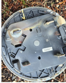
Back of electric meter. Notice corrosion on upper left connector
